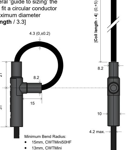
Standard 'Coil length' options are 100mm and 200mm though longer coils can be made to meet specific requirements.
