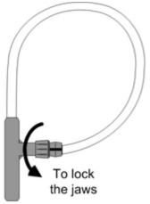
The locking mechanism must not be actuated at temperatures below 0°C
